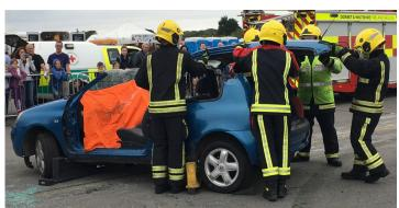
The Renault Clio's roof was cut off using massive hydraulic pincers.
