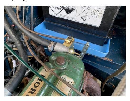
8. That's it. Choke cable should go over the heater hose, not be squashed under!
