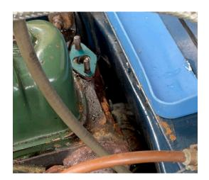
5. On OK but needed to be wiggled fairly forcibly down the studs. Getting the port/passenger side washer and nut on was an absolute fiddle. It's covered by the valve mechanism and therefore socket proof. I had no ratchet spanner and had to use a 7/16 AF open ended, turning over to grip the nuts 12 times for every turn. What a pain!
