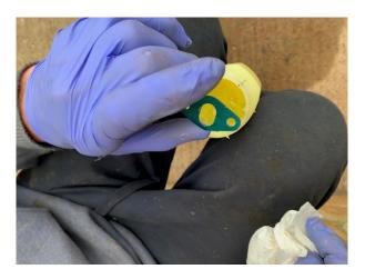
4. First mistake! The new gasket is not entirely symmetrical. The slightly thicker edge should be toward the front.
