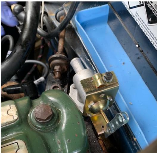
6. Nuts finally on and a pleasure to refit the hose - after freshening up the end by removing a couple of centimetres.
