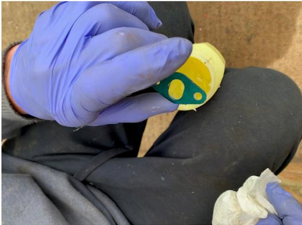
4. First mistake! The new gasket is not entirely symmetrical. The slightly thicker edge should be toward the front.
