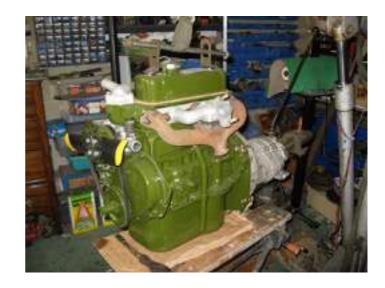
which looks correct with the Series II air cleaner modified with a K&N filter element so that it flows well and actually cleans the air! As 'Easy' was a 'base' model a heater was not present so a round style heater was fitted.
